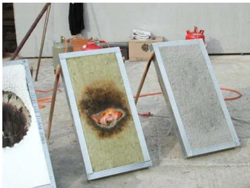
Links: PS-Dämmung B1,
