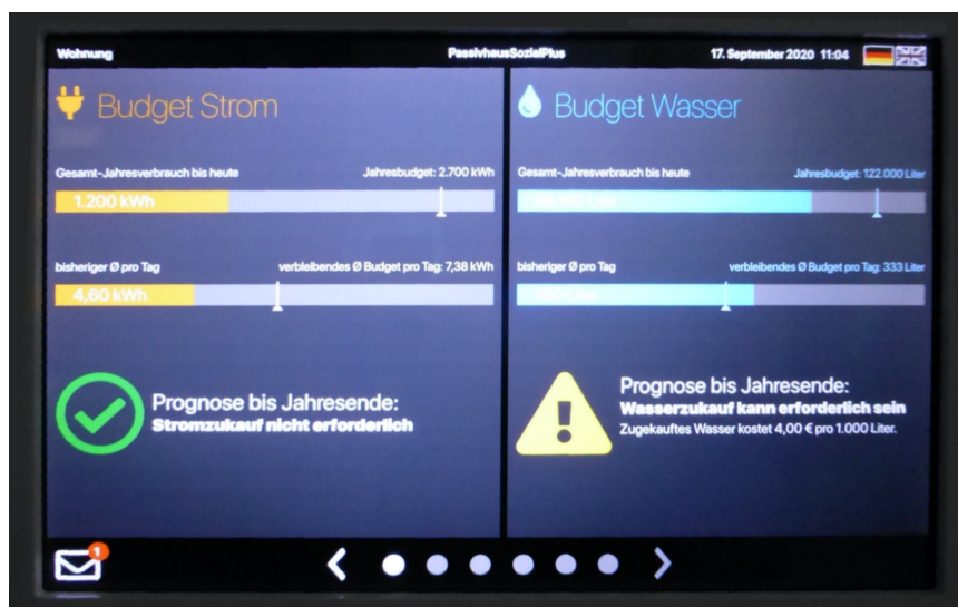
Figure 3. Overview page for consumption of electricity and drinking water on the display in a flat.
