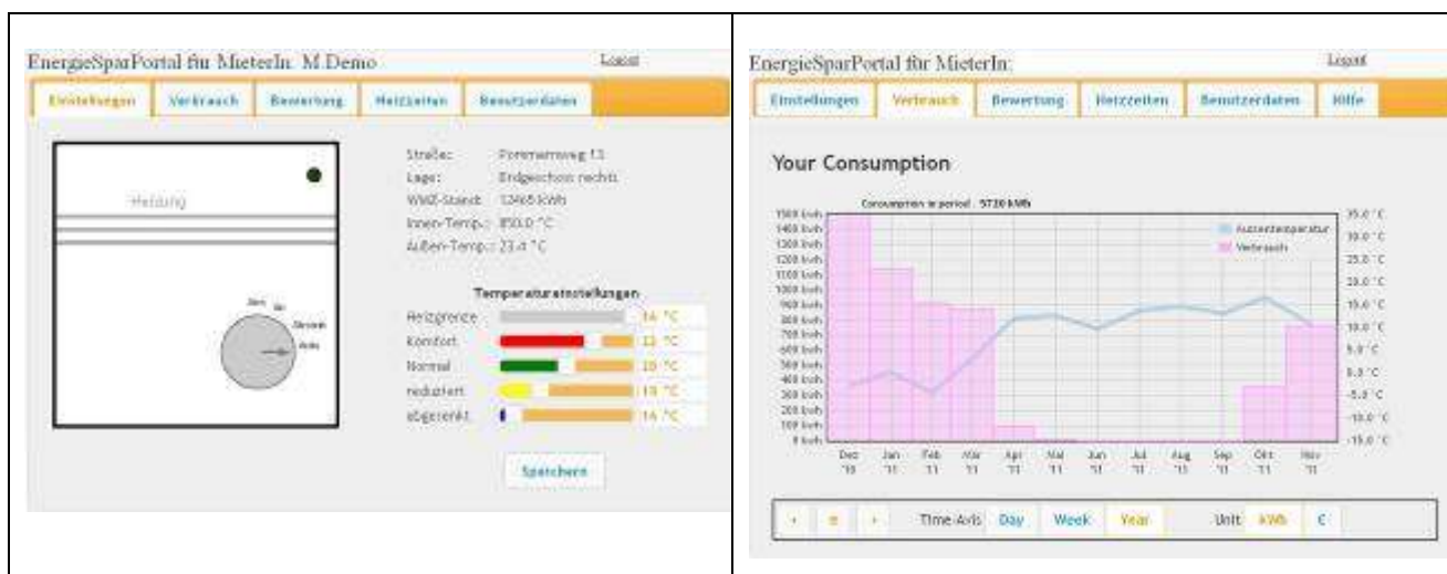
Figure 4-122: Screen shot of the EAS web portal (left: indoor temperature regulation for several, right: consumption feedback)
