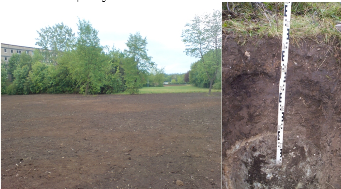
Fig. 3-8: New open space with homogenous soils and better ecological conditions – higher humus concentrations and thicker humic horizons
